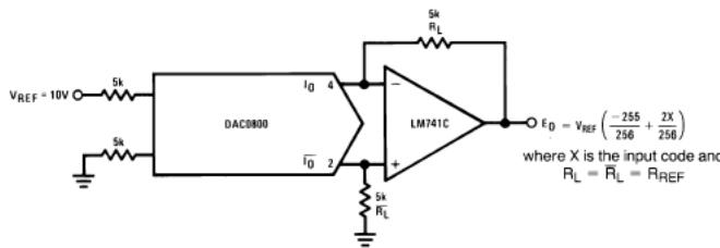
If  $R_L = \bar{R}_L$  within  $\pm 0.05\%$ , output is symmetrical about ground
