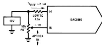
FIGURE 4. Recommended Full Scale Adjustment Circuit (Note 5)
