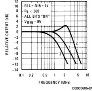
Curve 1:  $C_C = 15 \text{ pF}$ ,  $V_{IN} = 2 \text{ Vp-p}$  centered at 1V.
