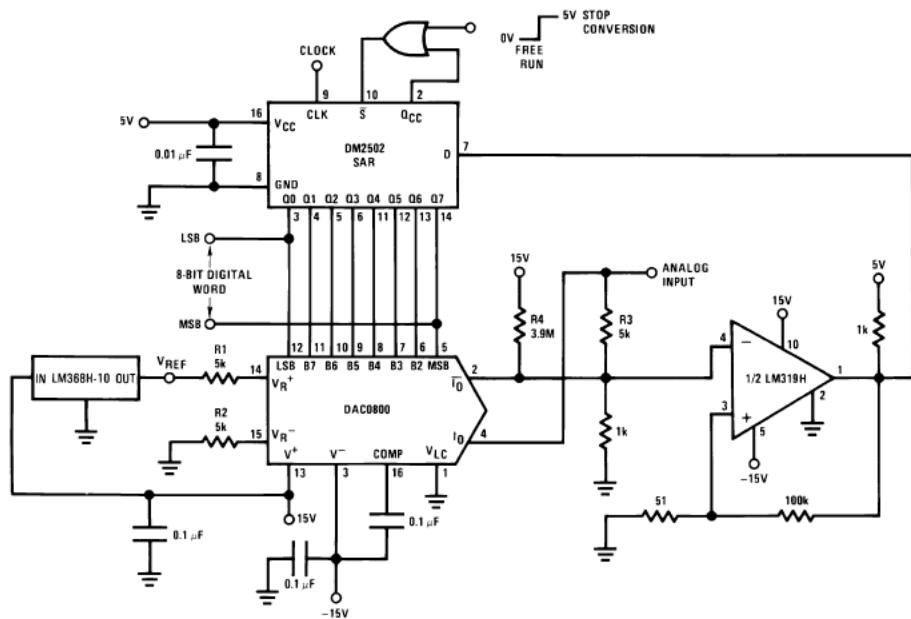
Note. For 1  $\mu$ s conversion time with 8-bit resolution and 7-bit accuracy, an LM361 comparator replaces the LM319 and the reference current is doubled by reducing R1, R2 and R3 to 2.5 k $\Omega$  and R4 to 2 M $\Omega$ .
