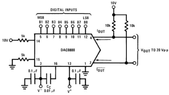
**FIGURE 1** ±20 V – Output Digital-to-Analog Converter (Note 5)
