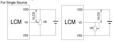
$V_{DD-V_0}$ : LCD Driving voltage VR: 10k~20k
