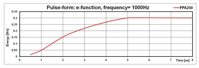
Whilst these parts are designed to operate in high frequency circuits, where dv/dt is faster than 250V/ $\mu$ S, it is recommended that the resistor is tested under worst case application conditions to ensure that unknown attribute of the application waveform are completely accounted for.
