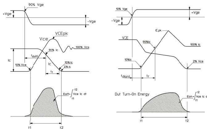
Fig. 22. Definition of switching times and losses
