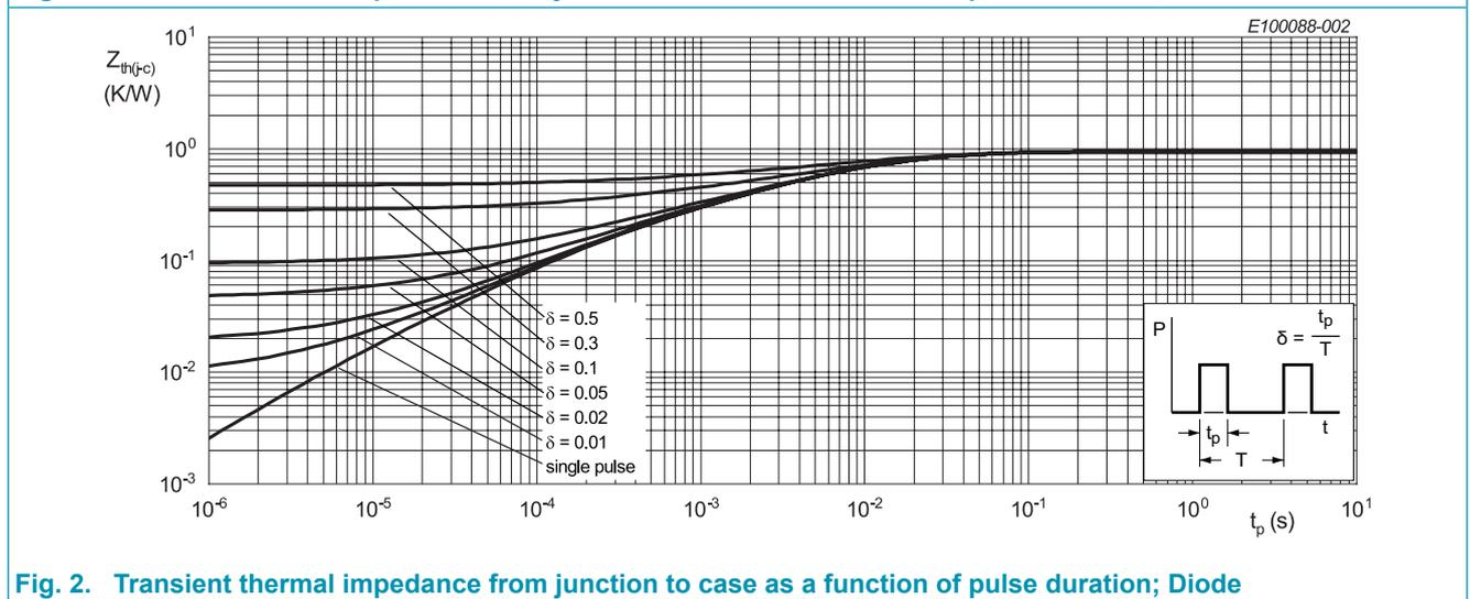
Fig. 2. Transient thermal impedance from junction to case as a function of pulse duration; Diode
