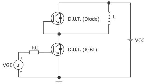
Fig. 21. Test circuit for inductive load switching
