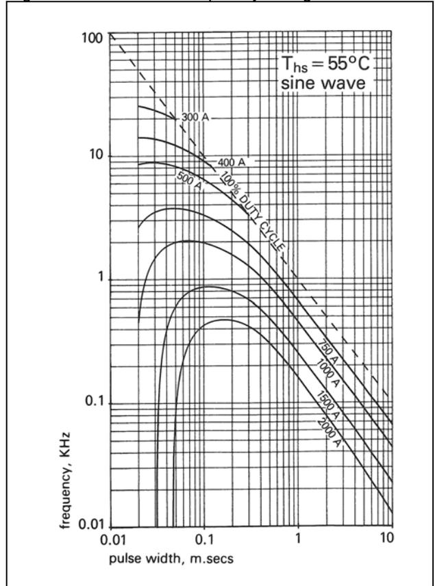
Figure 7 - Sine wave frequency ratings
