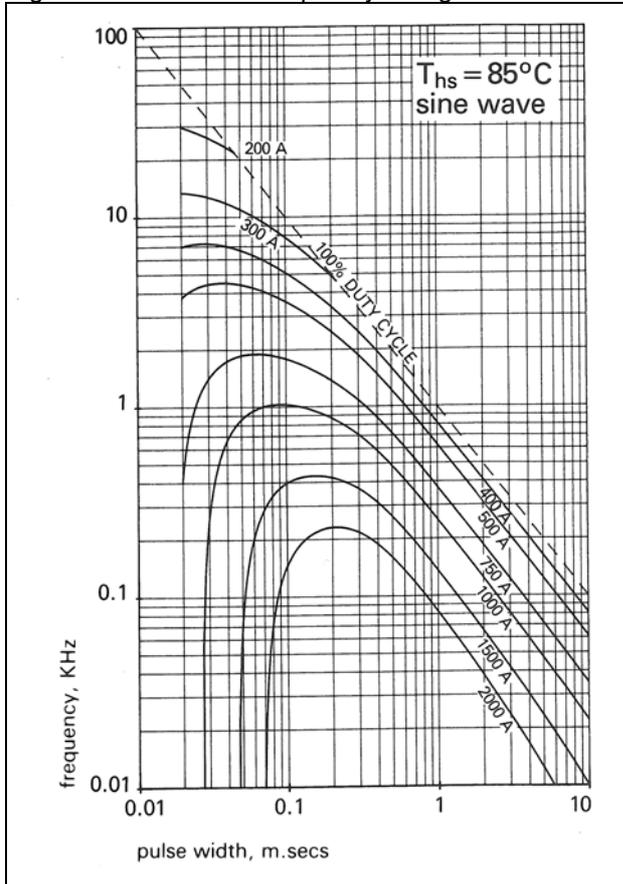
Figure 8 - Sine wave energy per pulse
