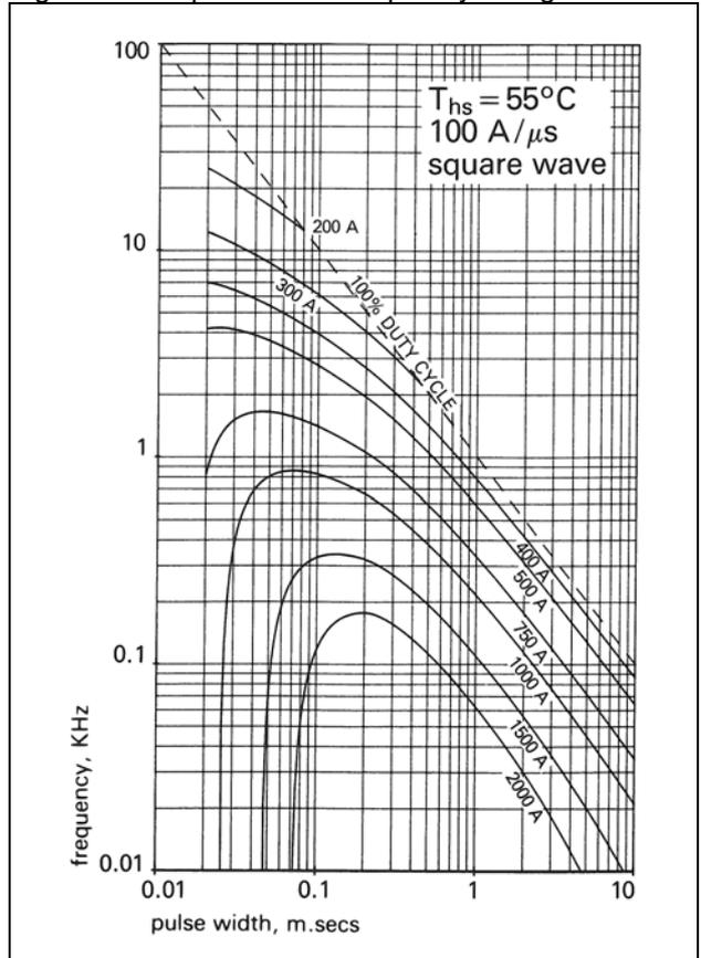
Figure 13 - Square wave energy per pulse
