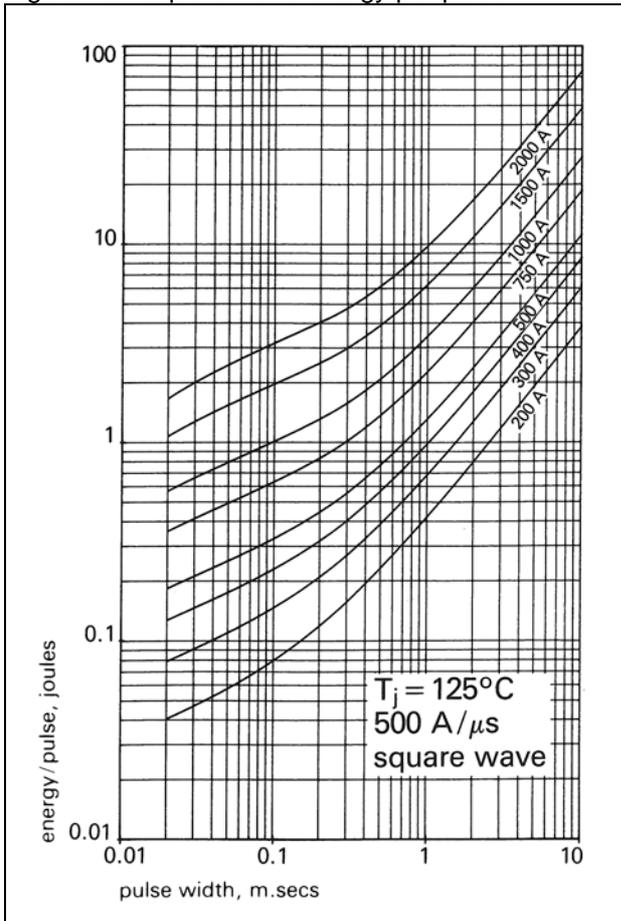
Figure 14 - Square wave energy per pulse
