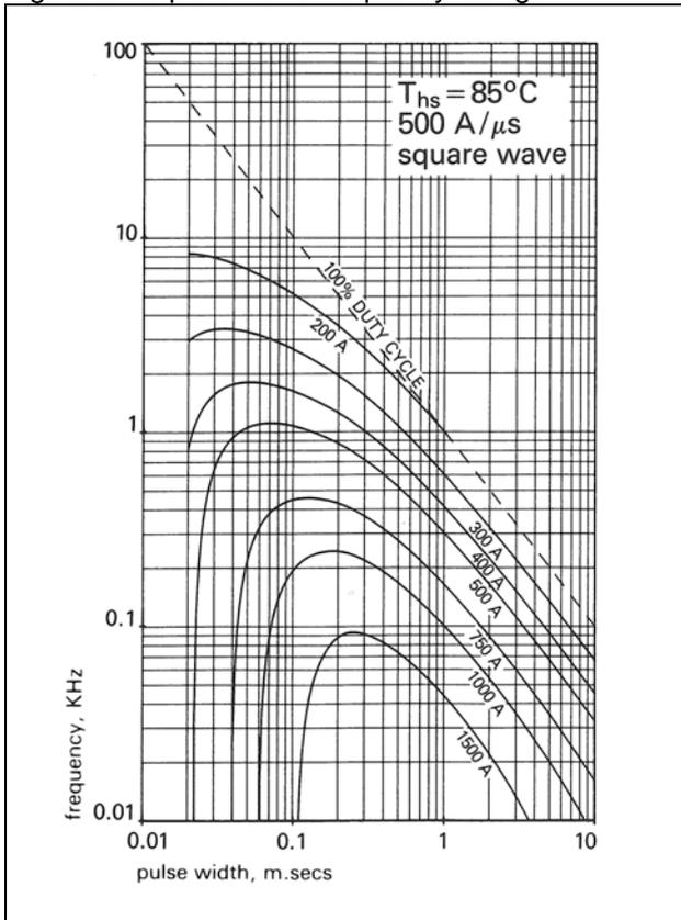
Figure 10 - Square wave frequency ratings
