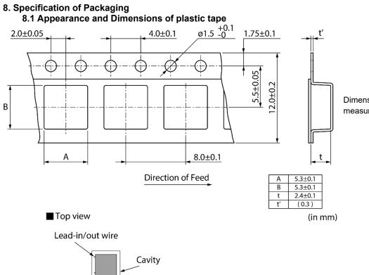
Dimension of the Cavity is measured at the bottom side.
