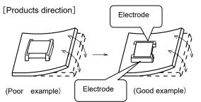
The electorode part of the products should be located like the picture to the mechanical stress.
