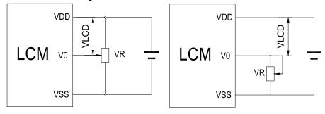
$V_{DD\sim}V_0$ : LCD Driving voltage
