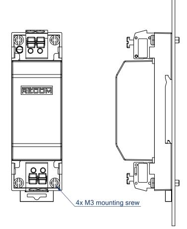
Recommended mounting tightening torque= 0.7Nm
