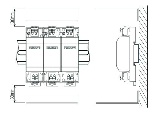
Note11: Panel mount installations can be realized in any orientation. No distance to adjacent components is required for thermally effective contact. In pure convection cooled ambient at least two of four long sides shall have access to air convection (eg 2cm distance)
