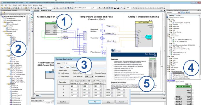
Figure 1. Multiple-Sensor Example Project in PSoC Creator
