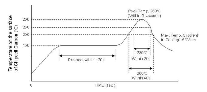
The time of repeated reflow soldering must be two times or less.
