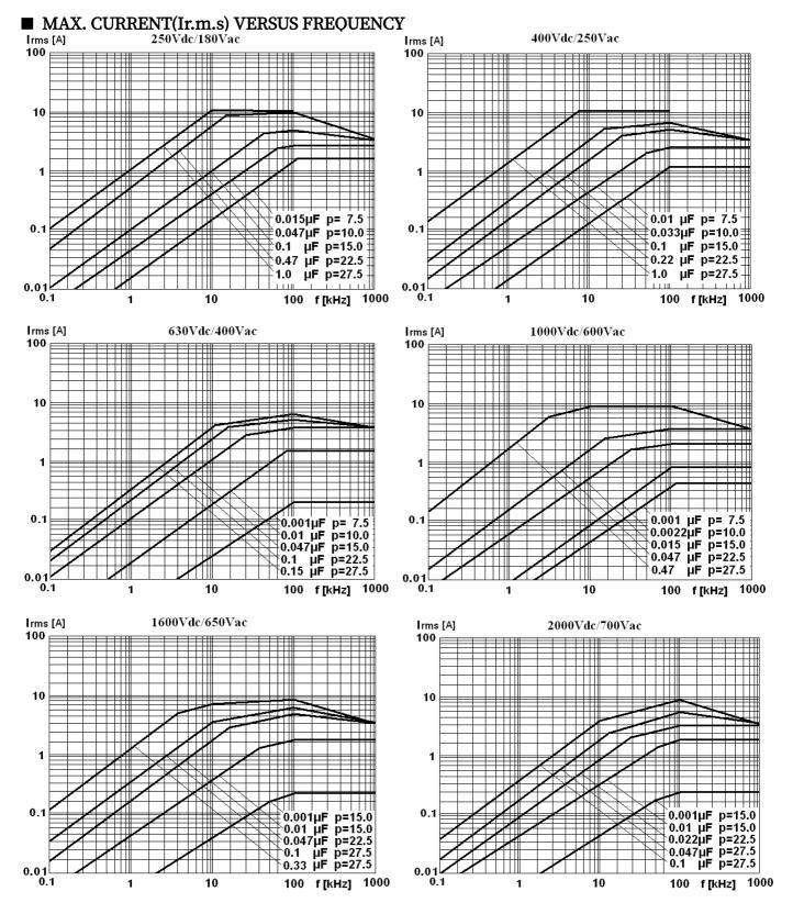
Note: sinusoidal wave-form, environment temperature  $\leq$  85°C, internal temperature rise  $\triangle$ T=10°C, p (pitch) in mm.
