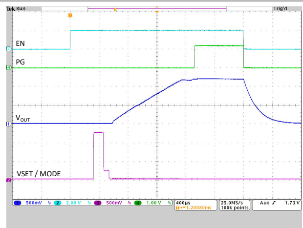
R_{VSET} = 56.2 \text{ k}\Omega I_{OUT} = 0 \text{ A} Figure 8-33. Start-Up with No Load
