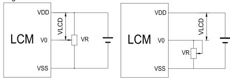
$V_{DD\sim}V_0$ : LCD Driving voltage
