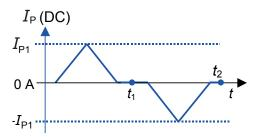
Figure 2: Current cycle used to measure magnetic and electrical offset (transducer supplied)
