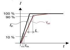
Figure 3: Response time  $t_r$  and reaction time  $t_{ra}$
