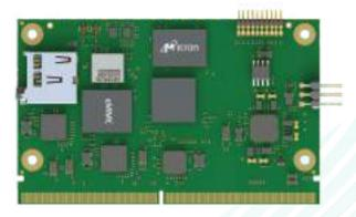
The i.MX 93 or i.MX 91 SoC based SMARC System On Module is designed as per SMARC specification v2.1.1. It integrates NXP's i.MX 93 offerings Dual Cortex A55 @ 1.7GHz, NPU with up to 0.5 TOP/s\* and IEEE 802.11 a/b/g/n/ac/ax Wi Fi + Bluetooth 5.3 module.
