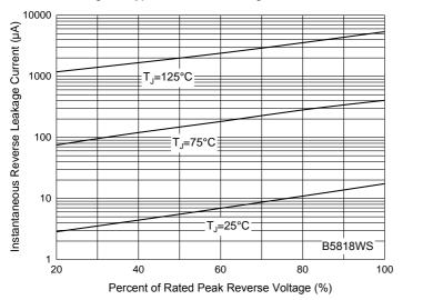
Fig. 7 - Typical Reverse Leakage Characteristics
