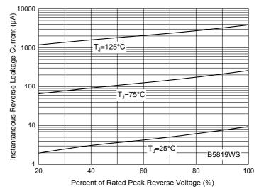
Fig. 8 - Typical Reverse Leakage Characteristics
