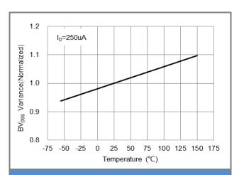
Fig.8 Breakdown Voltage Variation vs. Temperature
