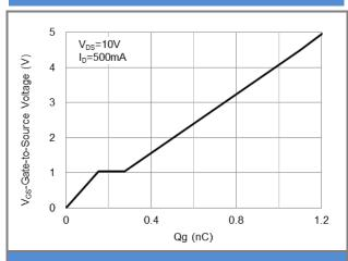
Fig.7 Gate-Charge Characteristics
