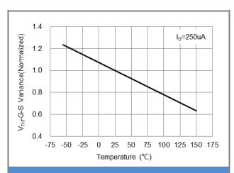
Fig.9 Threshold Voltage Variation with Temperature
