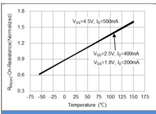
Fig.4 On-Resistance vs. Junction temperature
