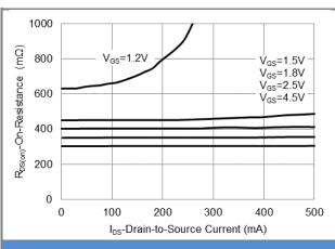
Fig.3 On-Resistance vs. Drain Current
