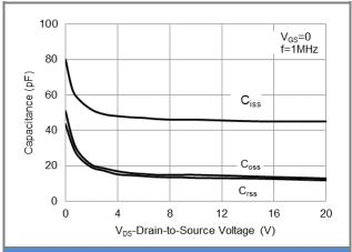
Fig.10 Capacitance vs. Drain-Source Voltage
