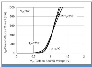
Fig.2 Transfer Characteristics
