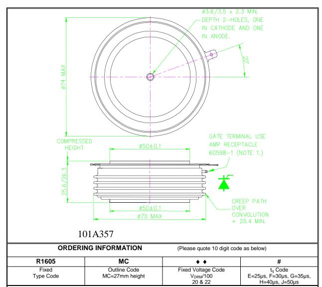
Typical order code: R1605MC22E - 2200V  $V_{DRM}$  and  $V_{RRM}$  25 $\mu$ s  $t_q$ , 26.3mm clamp height capsule
