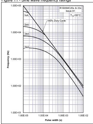
Figure 12 - Sine wave frequency ratings
