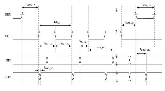
Fig.2.4.1 SPI Timing
