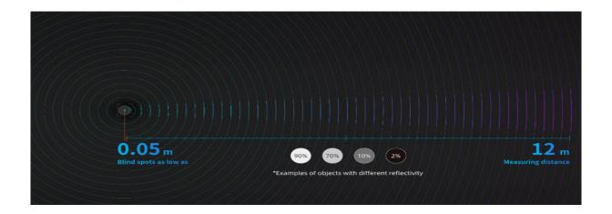
Its scanning frequency of 10Hz (600rpm) enables a sample rate of 5KHz and an angular resolution of 0.72°. It provides 2.5D multidimensional information, including position information data and reflectivity data.
