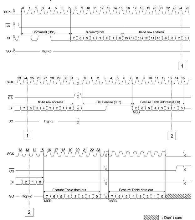
Figure 18. Block Erase Timing
