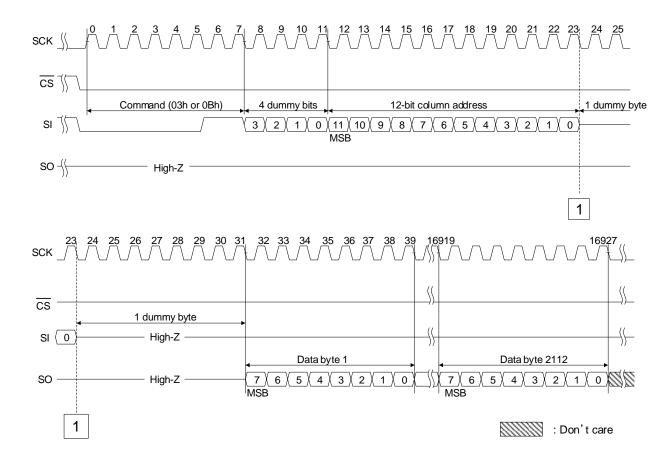
Note: When internal ECC is turned OFF, the maximum output data size is 2176 Bytes.
