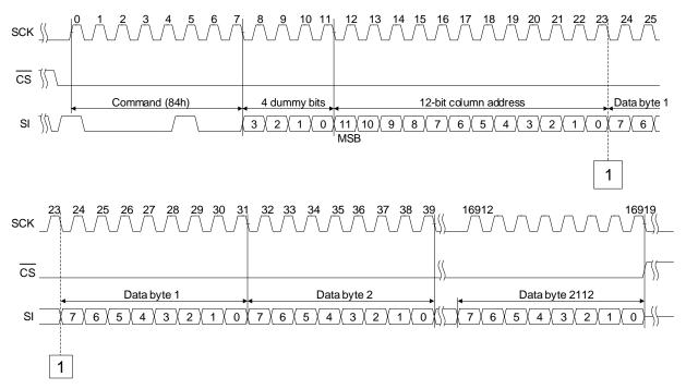
Note: When internal ECC is turned OFF, the maximum input data size is 2176 Bytes.
