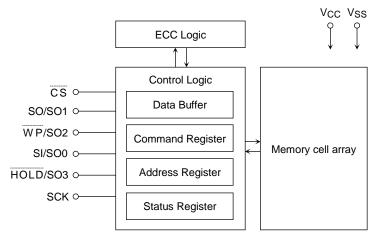
Figure 2. Block Diagram
