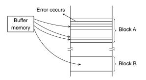
When an error happens in Block A, reprogramming the data into another Block (Block B) by loading from an external buffer. Then, prevent further system accesses to Block A (by creating a bad block table or by using another appropriate scheme).
