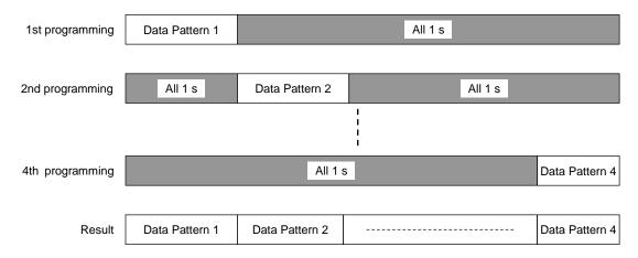
Program Load Random Data (84h) command can be used to skip column address within the selected page to improve the data input operation.
