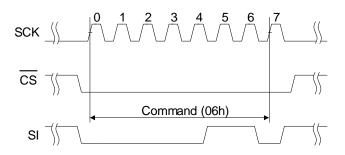
Figure 20. Write Enable Timing
