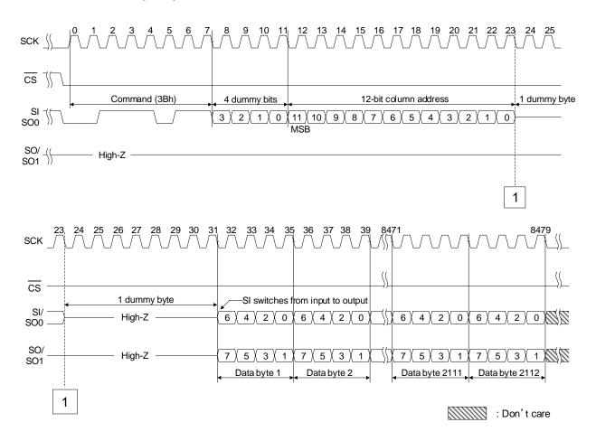
Note: When internal ECC is turned OFF, the maximum output data size is 2176 Bytes.
