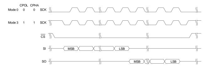
Figure 5. SPI Timing
