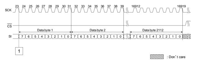
Note: When internal ECC is turned OFF, the maximum input data size is 2176 Bytes.
