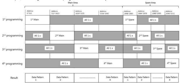
Program Load Random Data (84h) command can be used to skip column address within the selected page to improve the data input operation.
