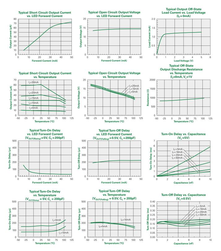
All temperatures are ambient and unless otherwise noted, the graph data is typical of the device at  $T_A = 25$ °C. Device performance illustrated in the Characteristic Curves beyond the maximum ambient operational temperature of 85°C are for informational purposes only and do not constitute or imply approval to operate the device beyond the ratings stated in the specifications.
