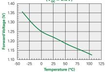
All temperatures are ambient and unless otherwise noted, the graph data is typical of the device at T<sub>A</sub> = 25°C. Device performance illustrated in the Characteristic Curves beyond the maximum ambient operational temperature of 85°C are for informational purposes only and do not constitute or imply approval to operate the device beyond the ratings stated in the specifications.
