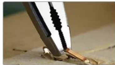
Pliers used as a Carton Staple Remover
