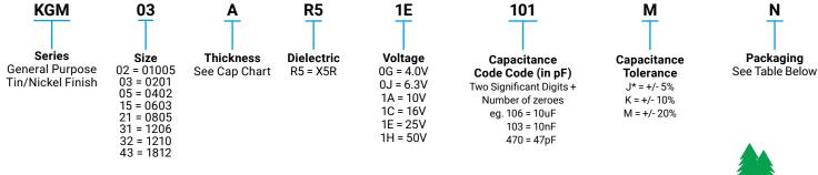
NOTE: Contact factory for availability of Tolerance Options for Specific Part Numbers. Contact factory for non-specified capacitance values.
