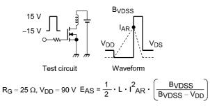
Fig. 8.16 Test Circuit/Waveform
