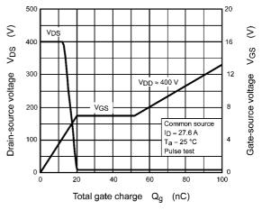
Fig. 8.12 Dynamic Input/Output Characteristics
