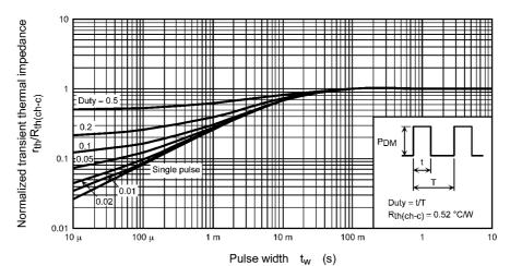
Fig. 8.13 r<sub>th</sub> - t<sub>w</sub> (Guaranteed Maximum)
