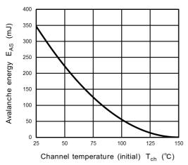
Fig. 8.14 E<sub>AS</sub> - T<sub>ch</sub> (Guaranteed Maximum)
