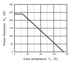
Fig. 8.15 P<sub>D</sub> - T<sub>c</sub> (Guaranteed Maximum)
