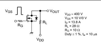
Fig. 6.2.1 Switching Time Test Circuit
