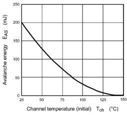
Fig. 8.14 E<sub>AS</sub> - T<sub>ch</sub> (Guaranteed Maximum)
