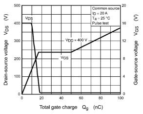
Fig. 8.12 Dynamic Input/Output Characteristics
