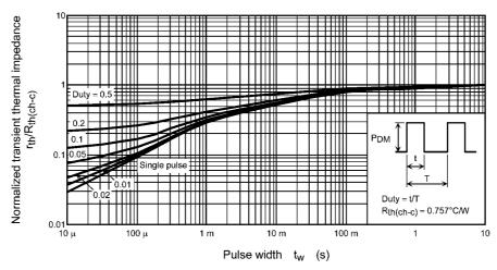
Fig. 8.13 r<sub>th</sub> - t<sub>w</sub> (Guaranteed Maximum)
