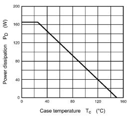
Fig. 8.15 P<sub>D</sub> - T<sub>c</sub> (Guaranteed Maximum)
