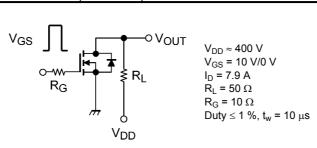
Fig. 6.2.1 Switching Time Test Circuit
