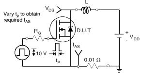
Fig. 16 - Unclamped Inductive Test Circuit
