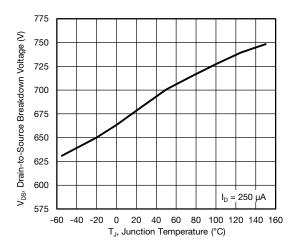
Fig. 11 - Temperature vs. Drain-to-Source Voltage
