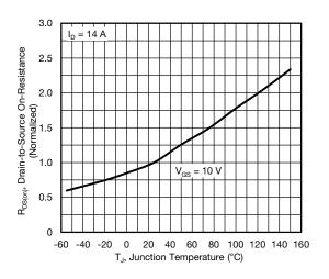
Fig. 4 - Normalized On-Resistance vs. Temperature
