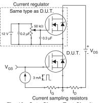
Fig. 19 - Gate Charge Test Circuit
