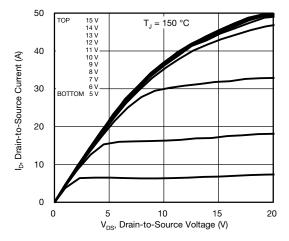
Fig. 2 - Typical Output Characteristics
