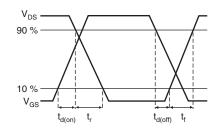
Fig. 15 - Switching Time Waveforms
