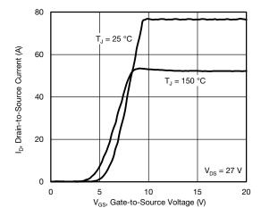
Fig. 3 - Typical Transfer Characteristics
