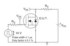
Fig. 14 - Switching Time Test Circuit
