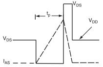
Fig. 17 - Unclamped Inductive Waveforms
