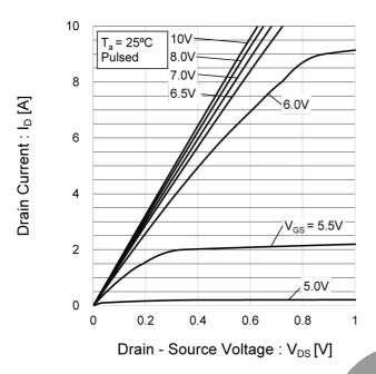
Fig.6 Typical Output Characteristics(II)
