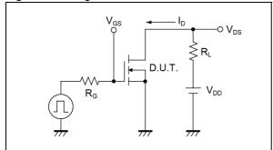
Fig.2-1 Gate Charge Measurement Circuit
