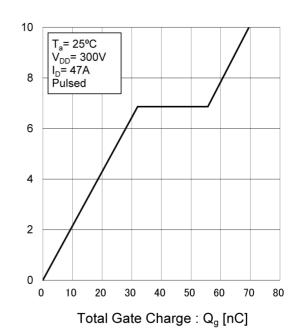
Gate - Source Voltage : V<sub>GS</sub> [V]
