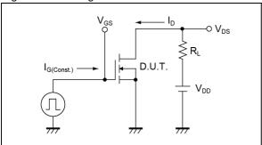
Fig.3-1 Avalanche Measurement Circuit
