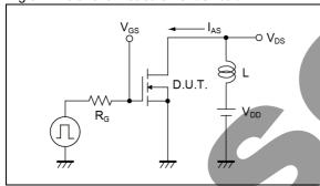
Fig.4-1 dv/dt Measurement Circuit
