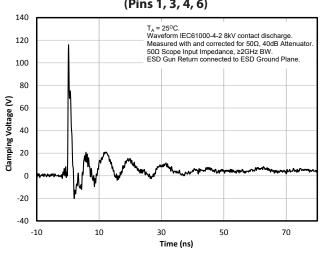
ESD Clamping (-8kV Contact per IEC 61000-4-2)
