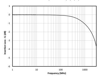
Insertion Loss (I/O Pin to I/O Pin)
