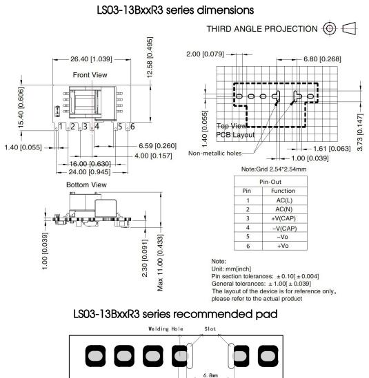
Note: There is a slot(non-metallic hole) between pin 4/5, which the side pad were being cut off. For details, please refer to the recommended dimensions or pad.
