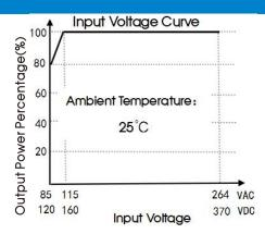
Note: ① With an AC input between 85-115VAC and a DC input between 120-160VDC, the output power must be derated as per temperature derating curves;
