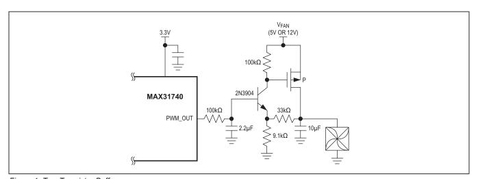
Figure 1. Two-Transistor Buffer
