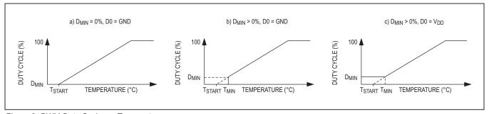
Figure 2. PWM Duty Cycle vs. Temperature
