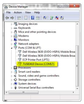
Figure 3. Device Manager with COM Port Name
