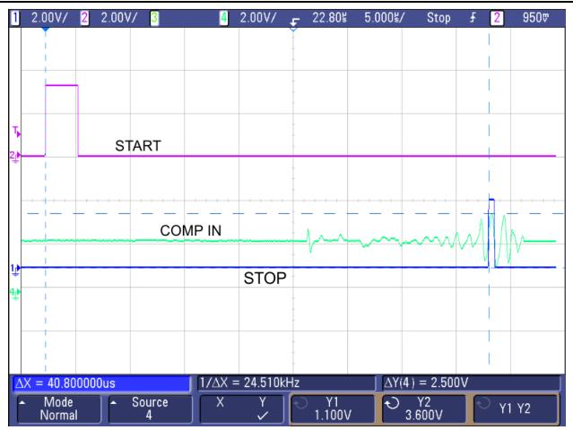
Figure 10. START, COMPIN and STOP Signals on Oscilloscope
