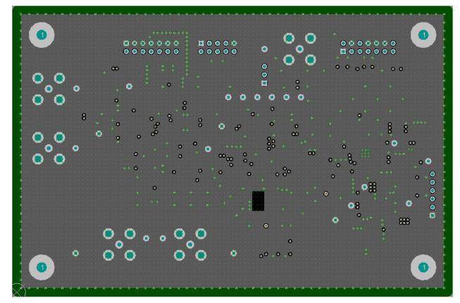
Figure 14. Ground Layer Routing
