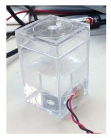
Figure 2. Water Container with 1-MHz Transducer
