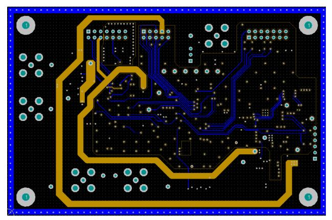
Figure 13. Power Layer Routing
