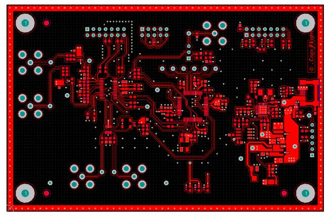
Figure 12. Top Layer Routing
