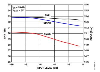
Figure 19. SNR, SINAD, and ENOB vs. Input Level
