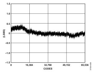
Figure 6. Integral Nonlinearity vs. Code
