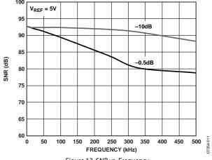
Figure 12. SNR vs. Frequency
