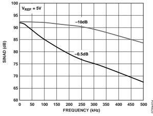
Figure 15. SINAD vs. Frequency
