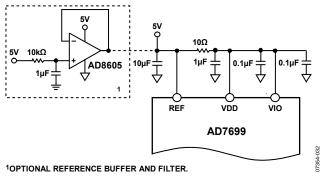
Figure 36. Example of an Application Circuit
