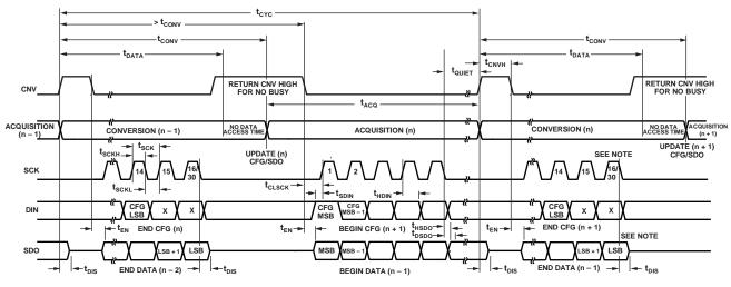
NOTES 1. THE LSB IS FOR CONVERSION RESULTS OR THE CONFIGURATION REGISTER CFG (n – 1) IF. 15 SCK FALLING EDGES = LSB OF CONVERSION RESULTS. 29 SCK FALLING EDGES = LSB OF CONFIGURATION REGISTER. ON THE 16TH OR 30TH SCK FALLING EDGE, SO IS DRIVEN TO HIGH IMPENDANCE. 2. NO DATA ACCESS TIME IS A DIFFERENCE BETWEEN  $t_{CONV}$  AND  $t_{DATA}$ .
