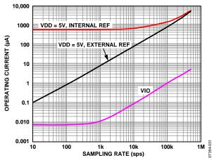
Figure 35. Operating Currents vs. Sampling Rate
