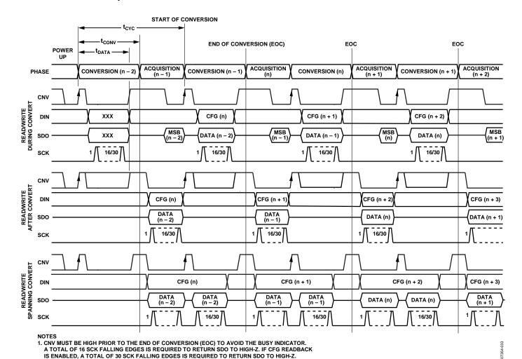
Figure 37. General Interface Timing for the AD7699 Without a Busy Indicator
