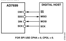
Figure 39. Connection Diagram for the AD7699 Without a Busy Indicator
