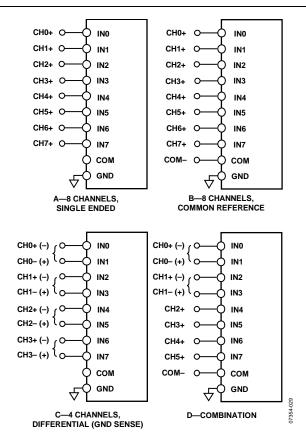
Figure 33. Multiplexed Analog Input Configurations
