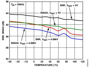
Figure 14. SNR, SINAD vs. Temperature
