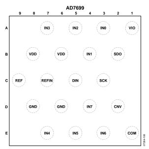
Figure 5. 20-Lead WLCSP Pin Configuration
