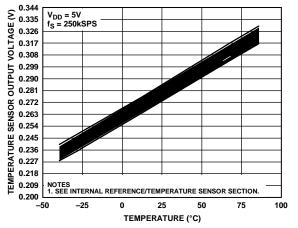
Figure 26. Temperature Sensor Output Voltage vs. Temperature
