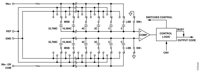
Figure 27. ADC Simplified Schematic
