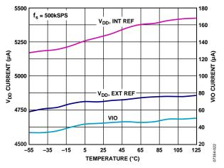
Figure 22. Operating Currents vs. Temperature
