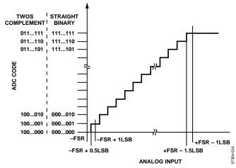
Figure 28. ADC Ideal Transfer Function
