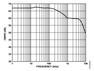
Figure 32. Analog Input CMRR vs. Frequency
