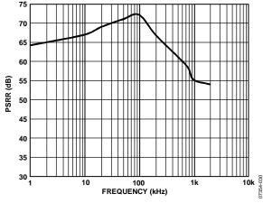
Figure 34. PSRR vs. Frequency
