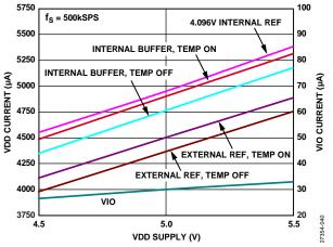
Figure 23. Operating Currents vs. Supply
