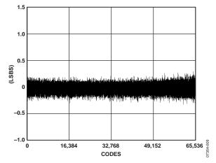
Figure 9. Differential Nonlinearity vs. Code
