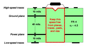
Figure 19. Recommended Layer Stack
