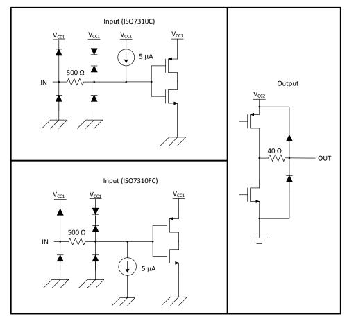
Figure 14. Device I/O Schematics
