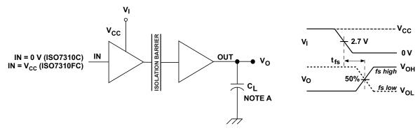
A.  $C_L = 15 \text{ pF}$  and includes instrumentation and fixture capacitance within ±20%.
