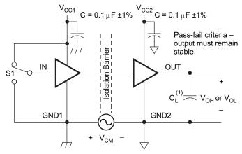
(1)  $C_L = 15 \text{ pF}$  and includes instrumentation and fixture capacitance within ±20%.
