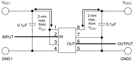
Figure 16. Typical ISO7310 Circuit Hook-up
