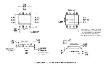
Figure 81. 8-Lead Standard Small Outline Package, with Exposed Pad [SOIC\_N\_EP]
