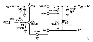
Figure 61. Typical Adjustable Output Voltage Application Schematic
