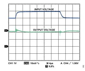
Figure 57. Line Transient Response,  $C_{IN}$  =  $C_{OUT}$  = 1  $\mu$ F,  $I_{LOAD}$  = 1 mA,  $V_{OUT}$  = 3.3 V
