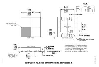
Figure 80. 8-Lead Lead Frame Chip Scale Package [LFCSP] 3 mm × 3 mm Body and 0.75 mm Package Height (CP-8-11)
