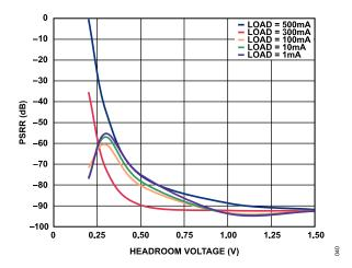
Figure 45. Power Supply Rejection Ratio (PSRR) vs. Headroom Voltage, 1 kHz,  $V_{OUT}$  = 5 V
