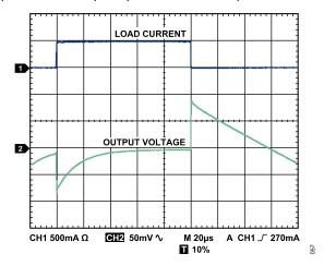
Figure 62. Output Transient Response,  $V_{OUT}$  = 1.8 V,  $C_{OUT}$  = 1  $\mu$ F
