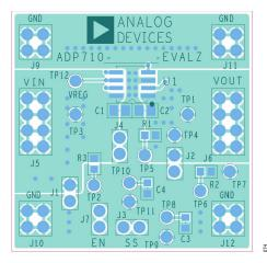
Figure 79. Example SOIC PCB Layout
