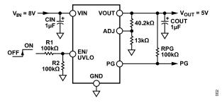
Figure 2. ADP7104 with Adjustable Output Voltage, 5 V
