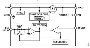
Figure 59. Fixed Output Voltage Internal Block Diagram
