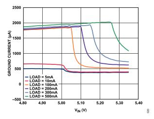
Figure 22. Ground Current ( $I_{GND}$ ) vs. Input Voltage ( $V_{IN}$ ) (in Dropout),  $V_{OUT} = 5 V$
