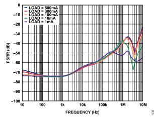
Figure 37. Power Supply Rejection Ratio (PSRR) vs. Frequency,  $V_{OUT}$  = 5 V,  $V_{IN}$  = 6.5 V
