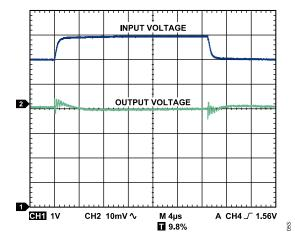
Figure 58. Line Transient Response,  $C_{IN}$  =  $C_{OUT}$  = 1  $\mu$ F,  $I_{LOAD}$  = 1 mA,  $V_{OUT}$  = 5 V
