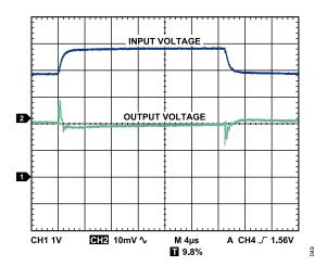
Figure 54. Line Transient Response,  $C_{IN}$  =  $C_{OUT}$  = 1  $\mu$ F,  $I_{LOAD}$  = 500 mA,  $V_{OUT}$  = 3.3 V
