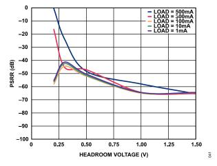
Figure 46. Power Supply Rejection Ratio (PSRR) vs. Headroom Voltage, 10 kHz, V<sub>OUT</sub> = 5 V
