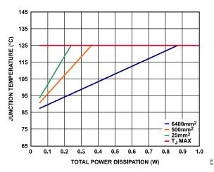
Figure 75. SOIC,  $T_A = 85$ °C
