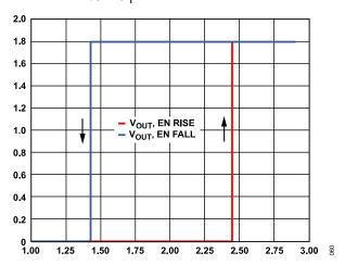
Figure 64. Typical VOUT Response to EN Pin Operation
