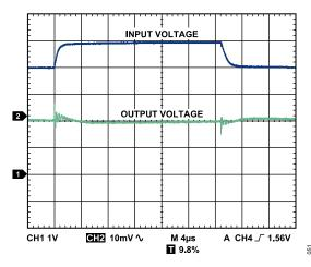
Figure 56. Line Transient Response,  $C_{IN}$  =  $C_{OUT}$  = 1  $\mu$ F,  $I_{LOAD}$  = 1 mA,  $V_{OUT}$  = 1.8 V
