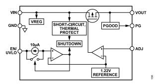
Figure 60. Adjustable Output Voltage Internal Block Diagram
