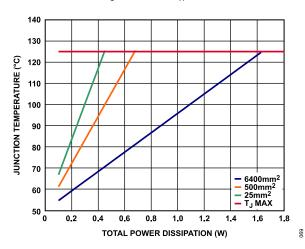
Figure 74. SOIC,  $T_A = 50$ °C
