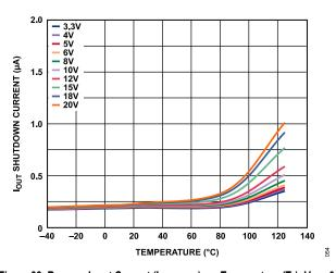
Figure 32. Reverse Input Current ( $I_{REV-INPUT}$ ) vs. Temperature ( $T_J$ ),  $V_{IN}$  = 0 V, Different Voltages on  $V_{OUT}$
