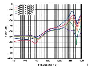
Figure 39. Power Supply Rejection Ratio (PSRR) vs. Frequency,  $V_{OUT}$  = 5 V,  $V_{IN}$  = 5.5 V
