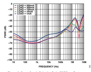
Figure 43. Power Supply Rejection Ratio (PSRR) vs. Frequency,  $V_{OUT}$  = 5 V,  $V_{IN}$  = 6 V, Adjustable with Noise Reduction Circuit
