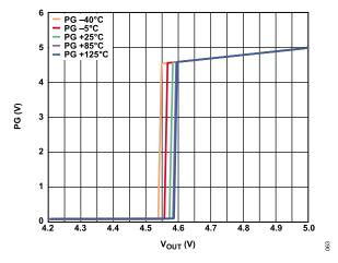
Figure 68. Typical Power-Good Threshold vs. Temperature, V<sub>OUT</sub> Falling
