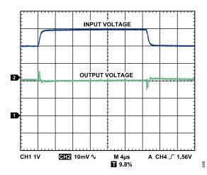
Figure 53. Line Transient Response,  $C_{IN}$  =  $C_{OUT}$  = 1  $\mu$ F,  $I_{LOAD}$  = 500 mA,  $V_{OUT}$  = 1.8 V
