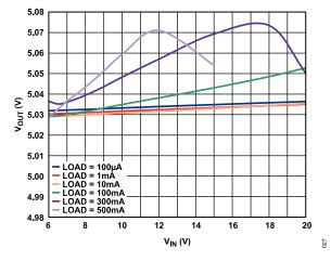
Figure 31. Output Voltage ( $V_{OUT}$ ) vs. Input Voltage ( $V_{IN}$ ),  $V_{OUT} = 5 V$ ,
