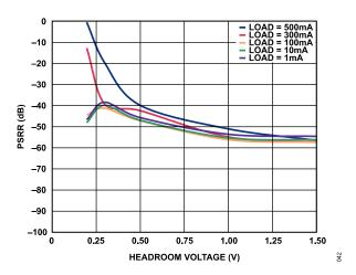
Figure 47. Power Supply Rejection Ratio (PSRR) vs. Headroom Voltage, 100 kHz,  $V_{OUT}$  = 5 V
