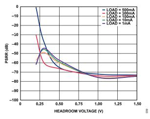
Figure 44. Power Supply Rejection Ratio (PSRR) vs. Headroom Voltage,  $100 \text{ Hz}, V_{OUT} = 5 \text{ V}$
