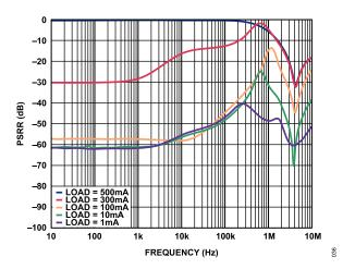
Figure 41. Power Supply Rejection Ratio (PSRR) vs. Frequency,  $V_{OUT} = 5 \text{ V}, V_{IN} = 5.2 \text{ V}$
