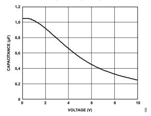
Figure 63. Capacitance vs. Voltage Characteristic
