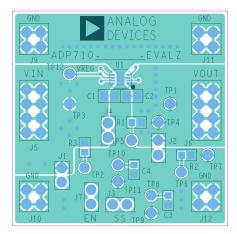
Figure 78. Example LFCSP PCB Layout
