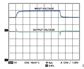
Figure 55. Line Transient Response,  $C_{IN}$  =  $C_{OUT}$  = 1  $\mu$ F,  $I_{LOAD}$  = 500 mA,  $V_{OUT}$  = 5 V
