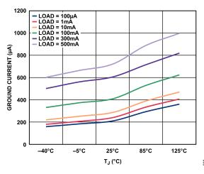
Figure 8. Ground Current ( $I_{GND}$ ) vs. Junction Temperature ( $T_{J}$ ),  $V_{OUT}$  = 3.3 V
