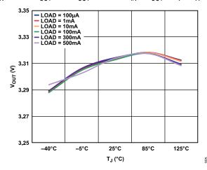
Figure 5. Output Voltage ( $V_{OUT}$ ) vs. Junction Temperature ( $T_J$ ),  $V_{OUT}$  = 3.3 V
