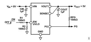
Figure 1. ADP7104 with Fixed Output Voltage, 5 V
