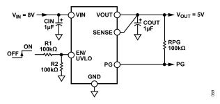
Figure 65. Typical EN Pin Voltage Divider
