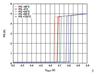
Figure 67. Typical Power-Good Threshold vs. Temperature, V<sub>OUT</sub> Rising
