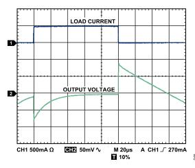
Figure 50. Load Transient Response,  $C_{IN}$  =  $C_{OUT}$  = 1  $\mu$ F,  $I_{LOAD}$  = 1 mA to 500 mA,  $V_{OUT}$  = 1.8 V,  $V_{IN}$  = 5 V
