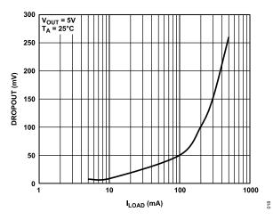
Figure 20. Dropout Voltage ( $V_{DROPOUT}$ ) vs. Load Current ( $I_{LOAD}$ ),  $V_{OUT} = 5 \text{ V}$
