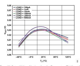
Figure 29. Output Voltage ( $V_{OUT}$ ) vs. Junction Temperature ( $T_J$ ),  $V_{OUT}$  = 5 V, Adjustable
