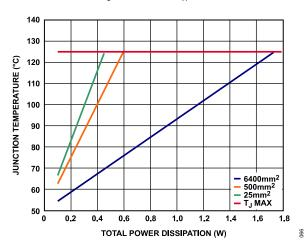
Figure 71. LFCSP, T<sub>A</sub> = 50°C
