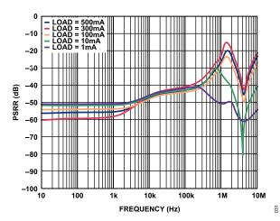
Figure 36. Power Supply Rejection Ratio (PSRR) vs. Frequency,  $V_{OUT}$  = 3.3 V,  $V_{IN}$  = 3.8 V
