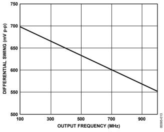
Figure 11. LVDS Differential Output Swing vs. Frequency
