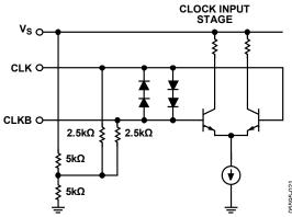
Figure 17. Clock Input Equivalent Circuit
