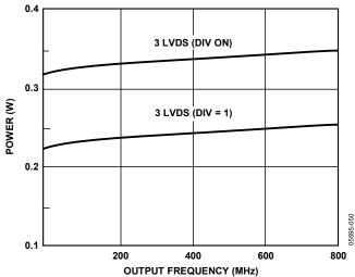
Figure 6. Power vs. Frequency—LVDS
