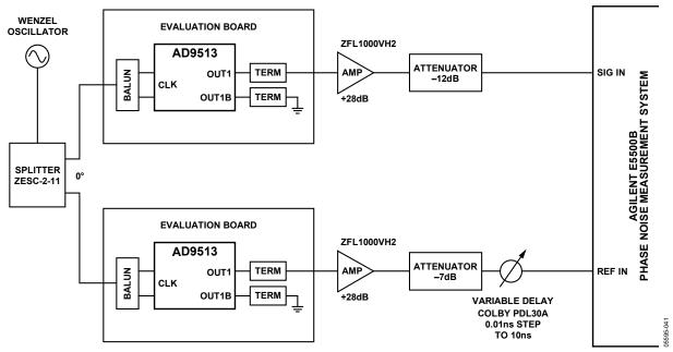
Figure 32. Additive Phase Noise Measurement Configuration
