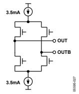
Figure 25. LVDS Output Simplified Equivalent Circuit
