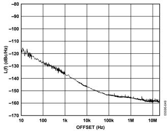
Figure 15. Additive Phase Noise—LVDS DIV2, 122.88 MHz
