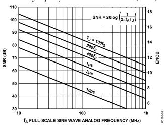
Figure 28. ENOB and SNR vs. Analog Input Frequency
