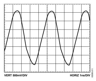
Figure 10. CMOS Single-Ended Output at 250 MHz with 10 pF Load
