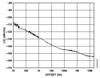
Figure 13. Additive Phase Noise—LVDS DIV 1, 245.76 MHz
