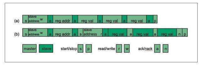
A typical *write* transaction (see Figure 16) therefore has the following format. The master initiates a transaction with a so-called start condition "s". This blocks the bus. Next, the master sends the 7 bits TH09 *slave address* followed by a 1 bit direction (a 0 indicating write "w"). This byte is acknowledged "a" by the slave. The master continues by sending the 8 bit register address, which is acknowledged by the slave.
