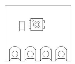
Relative Humidity and Temperature Sensor with I<sup>2</sup>C Interface
