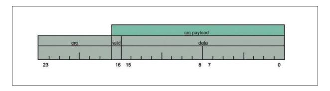
The *checksum* is a cyclic redundancy check over the data and the valid flag; the stored checksum is the result of CRC-7 (polynomial x7+x3+1, see *https://en.wikipedia.org/wiki/Cyclic\_redundancy\_check*) with 0x7F as initial vector (*i.e. with all bits flipped*), see Computing CRC-7 for sample C code.
