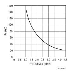
Figure 1. Frequency vs R<sub>T</sub>
