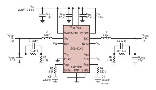
L1: MIDCOM DUS-5121-1R5R C<sub>OUT1</sub>: KEMET C1210C226K8PAC L2: MIDCOM DUS-5121-2R2R C<sub>OUT2</sub>, C<sub>IN</sub>: KEMET C1206C106K4PAC
