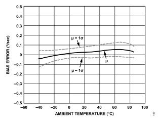
Figure 17. ADIS16477-3 Gyroscope Bias Error vs. Ambient Temperature
