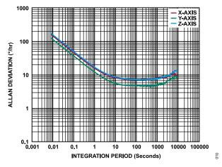
Figure 10. Gyroscope Allan Deviation, T<sub>C</sub> = 25°C, ADIS16477-3
