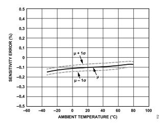
Figure 12. ADIS16477-1 Gyroscope Sensitivity Error vs. Ambient Temperature
