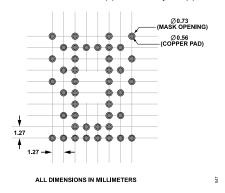
Figure 51. Recommend PCB Pattern, Solder Mask Defined Pads
