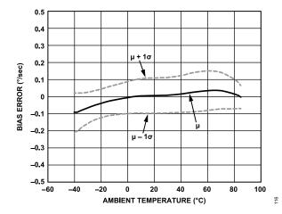
Figure 16. ADIS16477-2 Gyroscope Bias Error vs. Ambient Temperature
