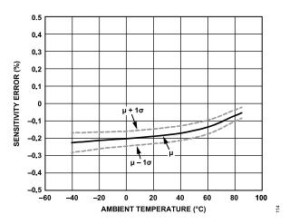
Figure 14. ADIS16477-3 Gyroscope Sensitivity Error vs. Ambient Temperature
