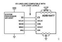
Figure 25. Electrical Connection Diagram
