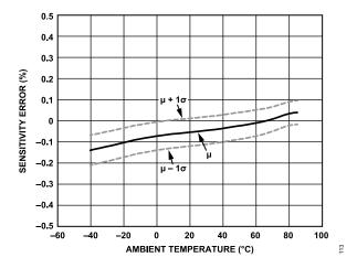
Figure 13. ADIS16477-2 Gyroscope Sensitivity Error vs. Ambient Temperature
