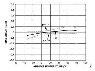
Figure 15. ADIS16477-1 Gyroscope Bias Error vs. Ambient Temperature
