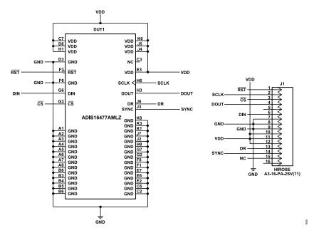
Figure 53. Breakout Board Schematic
