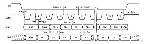
Figure 2. SPI Timing and Sequence Diagram
