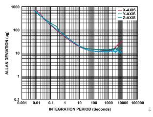
Figure 11. Accelerometer Allan Deviation, T<sub>C</sub> = 25°C
