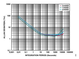
Figure 9. Gyroscope Allan Deviation,  $T_C$  = 25°C, ADIS16477-2
