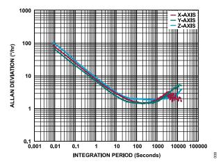
Figure 8. Gyroscope Allan Deviation, T<sub>C</sub> = 25°C, ADIS16477-1
