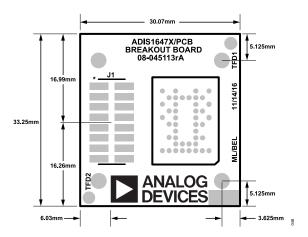
Figure 52. Top Level View of the Breakout Board
