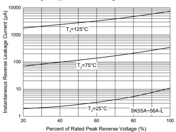
Fig. 8 - Typical Reverse Leakage Characteristics
