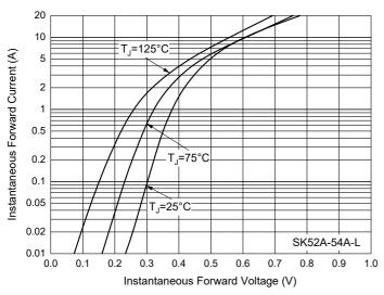
Fig. 5 - Typical Instantaneous Forward Characteristics
