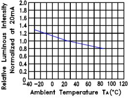
Fig.5 Relative Luminous Intensity VS. Ambient Temperature
