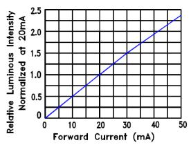
Fig.4 Relative Luminous Intensity vs. Forward Current
