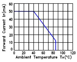
Fig.2 Forward Current Derating Curve
