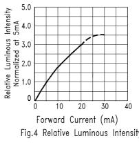
Fig.4 Relative Luminous Intensity vs. Forward Current
