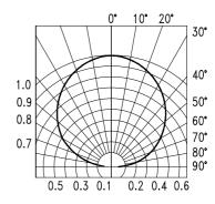
Fig.5 Luminous Intensity vs.
