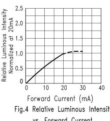
Fig.4 Relative Luminous Intensity vs. Forward Current
