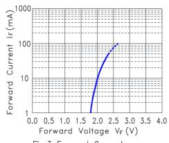
Fig.3 Forward Current vs. Forward Voltage
