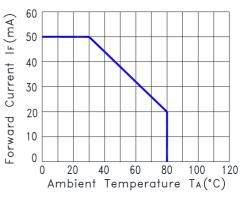
Fig.2 Forward Current Derating Curve
