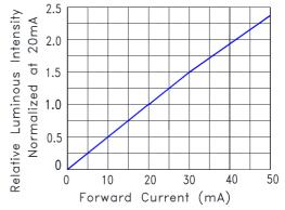
Fig.4 Relative Luminous Intensity vs. Forward Current
