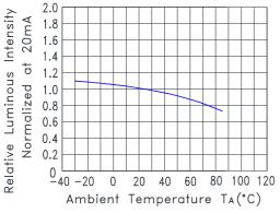
Fig.5 Relative Luminous Intensity VS. Ambient Temperature
