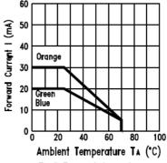
Fig.3 Forward Current Derating Curve
