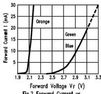
Fig.2 Forward Current vs. Forward Voltage
