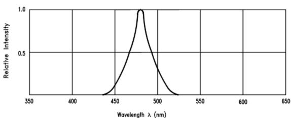
Fig.1 Relative Intensity vs. Wavelength
